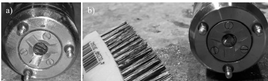
Figure 11. Scratches on fluorophore coating on OPT-sensor with iron brush. Scratches after 2 strokes in (a) and 5 additional strokes in (b).
