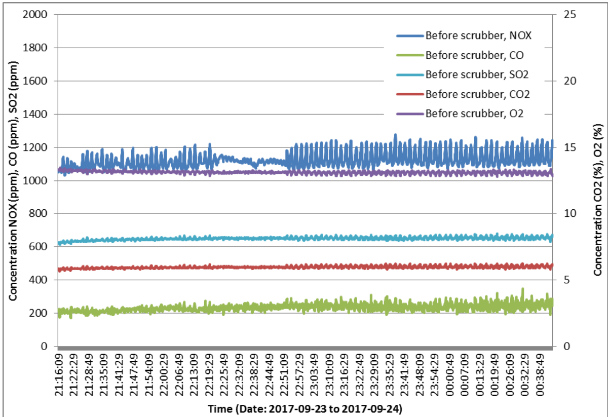
Figure B2. Gaseous emission concentrations of NO x , CO, CO 2 , O 2 , and SO 2 at 49% engine load, tests upstream the scrubber. Gas concentrations for time period 21:16:09 to 00:44:24 are used for further analysis
