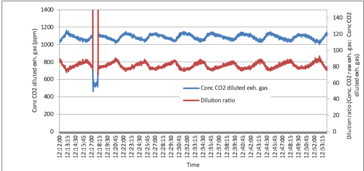
Figure A12. Dilution for sampling of filter 24. Concentrations of CO 2 in diluted gas and dilution ratio are shown. CO 2 in raw exhaust gas = 5.417%, CO 2 in ambient air = 420 ppm.
